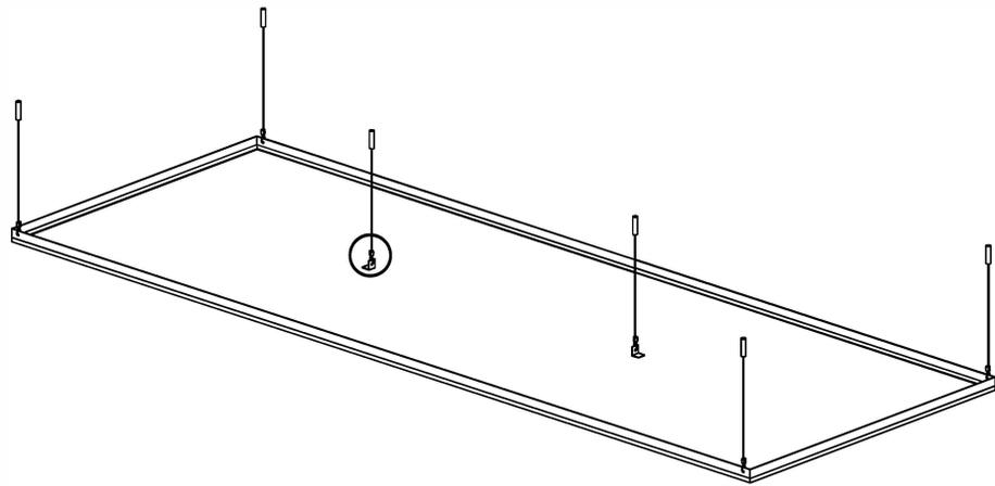
6. Adjust wire suspension height accordingly to ensure level hanging of screen.
